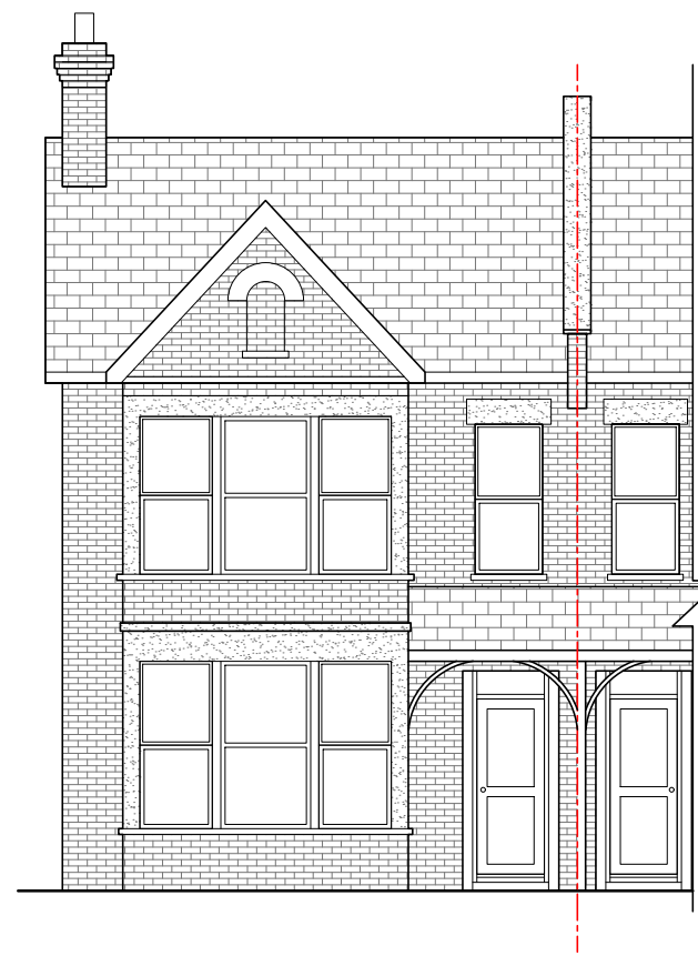
EXISTING FRONT ELEVATION SCALE 1:100 0 1 2 3 4 5m
