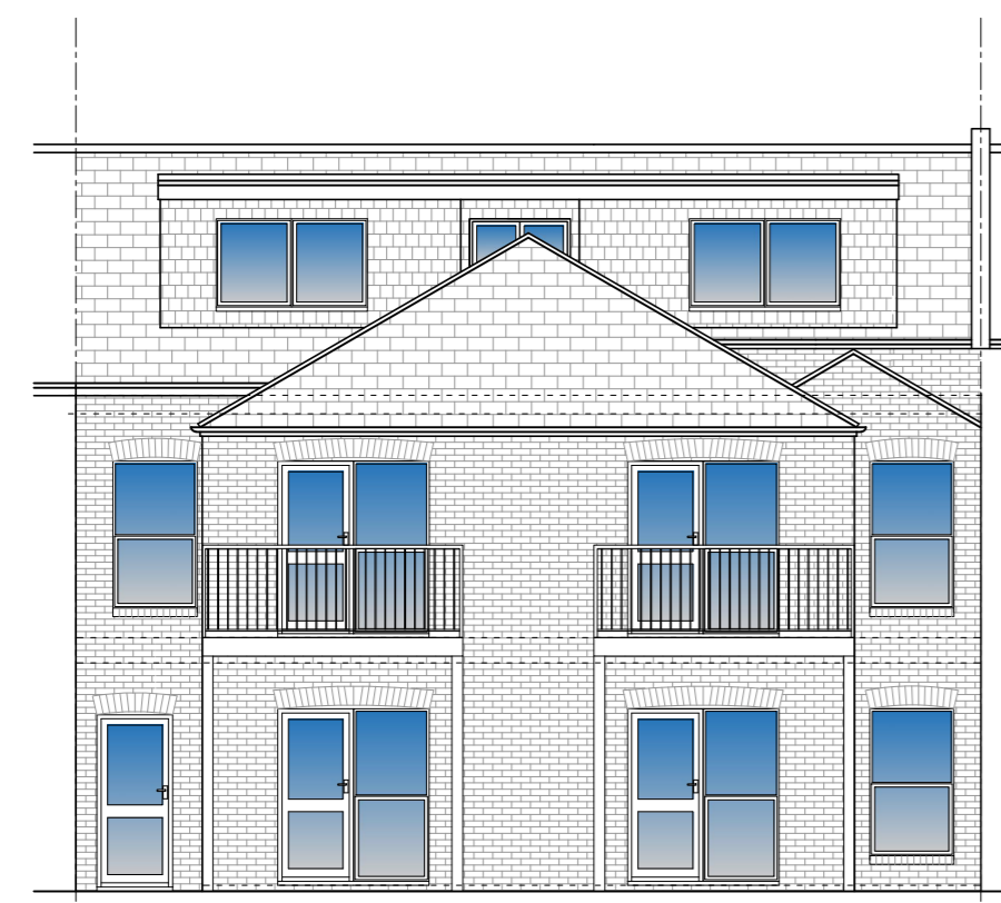
PROPOSED REAR ELEVATION SCALE 1:100 0 1 2 3 4 5m
